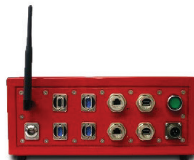
Digital I/O includes: 1 x Wireless 802.11b/g/n, 2 x Ethernet Ports, 2 USB Ports, 3 x Serial Ports (Upgradeable), and 1 x VGA Video
